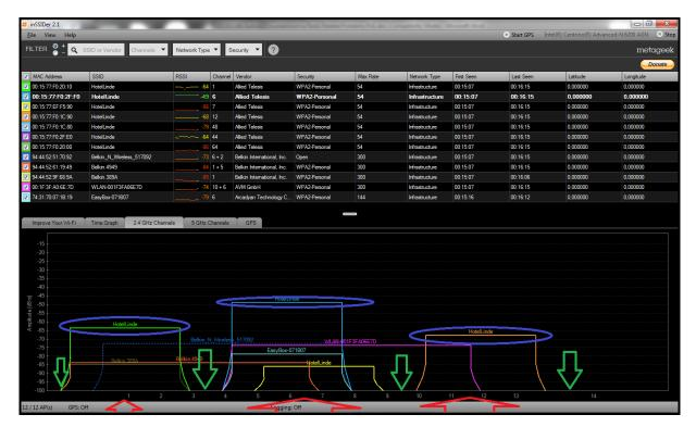
As the picture shows in this example, there are a number of different Wi-Fi networks in this particular surrounding. The signal strength varies in between them as shown with the blue markings. You can also see the channels used by those networks as shown with the red arrows. What is of interest now is to try to check channel overlap and possibly better channels to use. As you can see there are gaps in the overall 2.4 GHz band as shown with green arrows. This may be better choices for channels.
