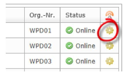
As soon as the gears have disappeared, load the firmware into all units in the second step. The gears then appear again and disappear after the firmware has been stored in the units.
