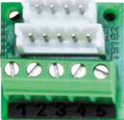
Connector Board Model 1385EAP SYSCON 4 / 5 Connector Board. Serves as an adapter to connect devices to SYSCON 4 or SYSCON 5 connecting cable. Connections are carried to screw terminals.
