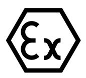
In rooms where natural gas, fuel or paint and solvent vapours are released, a single spark is enough to trigger explosions. All power-based devices (as well as electronic master key systems) must meet special requirements for hazardous areas. Ultimately, it comes down to suitable protective measures laid down in EU Directive 2014/34/EU, also known as ATEX 114 (ATmosphères EXplosibles). The ATEX guidelines provide extensive support for implementation.
