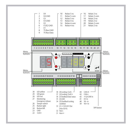
**DIP switch**All switches are set to the OFF position by the factory
