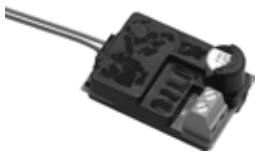
Pre-Load Electronic Assembly 760-12 Improves pre-load capability to at least 300N for DC operation. A short buzzing sound is audible in the electric strike for about 0.5 seconds. Continuous current-resistant, holding current is reduced. Compatible with standard effeff electric strikes
