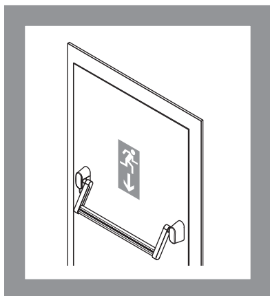
Fig. 5: A panic push bar according to EN 1125
